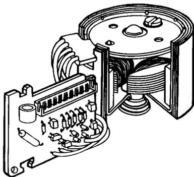
Clarion's dc servo motor assembly.
