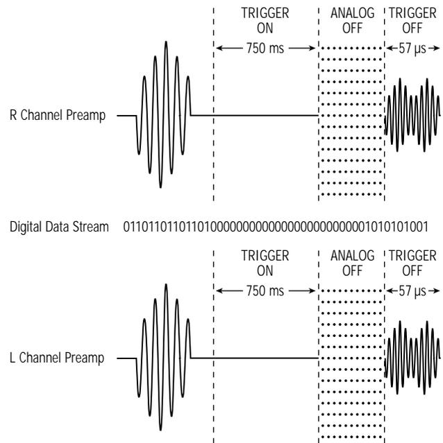
*The zero-bit detector mutes the preamplifier analog outputs after a series of zero bits exceeds 750 ms. Audio is restored after a period of one and zero bits is longer than 57 μ*
